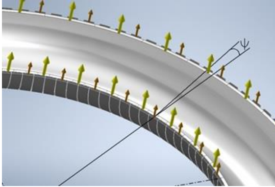
Figure 1 – Distribution of efforts in the torus tank in a meridional section
