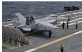
Figure 11 – F-18 Hornet ready for launch with electromagnetic catapult [20]
