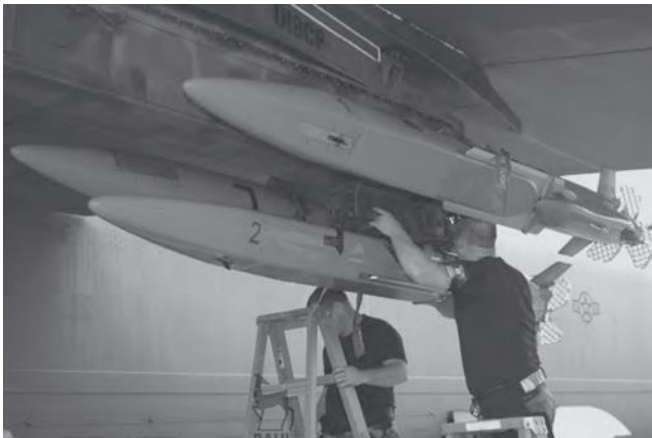
Figure 9 – The installation of the ADM-160B false radar target
