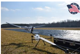
Figure 10 – MAAS 90 started with pneumatic launcher [19]
