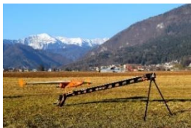
Figure 9 – Elastic launcher with a drone on it [18]
